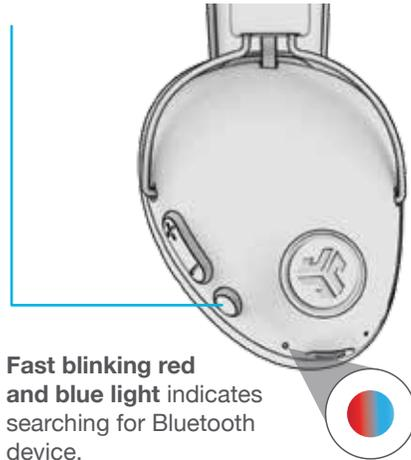
Fast blinking red and blue light indicates searching for Bluetooth device.
