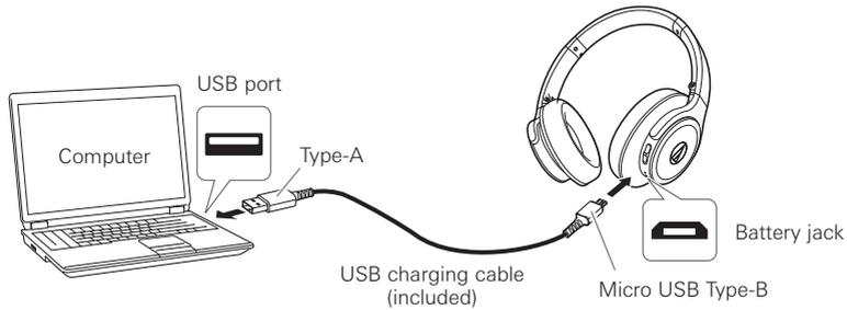
2. Connect the included USB charging cable (USB Type-A side) to the computer to start charging.
