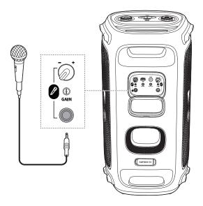
Connect a microphone to the microphone socket.
