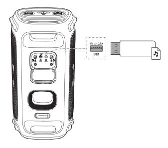
Plug a USB storage device that contains playable audio contents into the USB port of the speaker.
